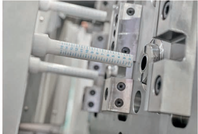
Fig. 3. The handling system moves into the mold (left) to place the labels in the eight cavities. Maximum precision is required to ensure that the scale reliably fulfills its purpose in the intended application. © Arburg
