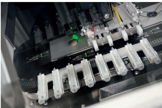
Fig. 4. The IMLWatcher is a complete solution for optical inspection of molded parts. The hardware is combined with software that is designed exclusively to detect IML-specific defects. © Arburg
