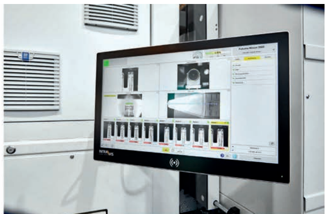
Fig. 4. The IMLWatcher is a complete solution for optical inspection of molded parts. The hardware is combined with software that is designed exclusively to detect IML-specific defects. © Arburg
